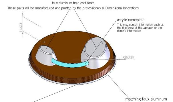
5 layers of 5/8-inch thick plywood, treated to match the benches found in Eaton Hall
