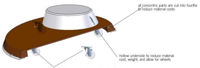
four casters will be housed inside the base to allow for transportation and will elevate the entire base by 1/4-inch
